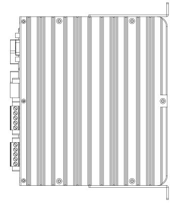
Figure 2.3. Rear Panel Mounting
